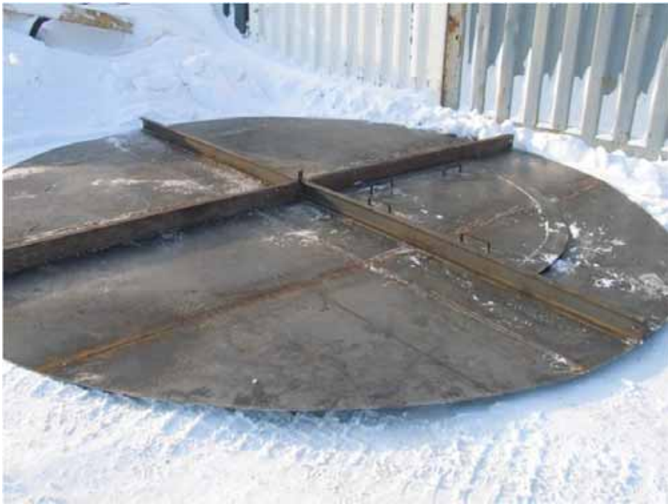
Photo 4: Fabricated sump lid
